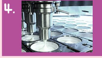
For fruit-on-the-bottom flavors, fruit is dispensed into the cups before the yogurt is added. The cups are sealed with foils and coded before being packed into cases and cooled.
