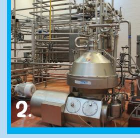
When milk arrives at the processing plant, a separator removes the cream from the milk and then the milk is reblended into skim, low fat, and whole categories.
