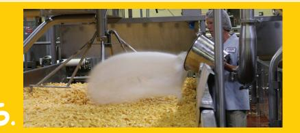
Salt and other ingredients for specialty cheese are added to the curds. Machines pack the curds into large blocks of cheese, which are then aged in a temperature-controlled warehouse.
