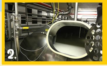
After the milk is trucked to the cheese processing plant, it is pasteurized, then poured into a cooking vat, where "good" bacteria are added as the milk is heated, allowing the bacteria to grow.
