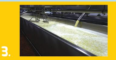
A special enzyme called rennet is added to the milk, which helps the "good" bacteria cause a chemical reaction that separates the milk proteins into liquids (whey) and solids (curds).
